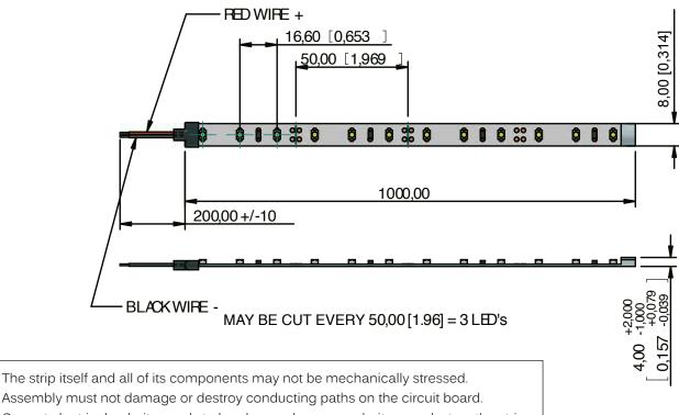
Correct electrical polarity needs to be observed, wrong polarity may destroy the strip. When mounting on a metallic or otherwise conductive surfaces, there needs to be electrical isolation points between strip and the mounting surface.
