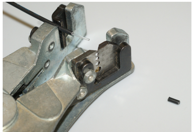
Figure 20. POF cable stripping using Ideal strip-master
