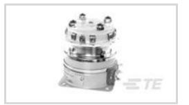
Power Relay Type: Rotary Coil Magnetic System: Non-Latching Coil Power Rating DC: 10300 mW Coil Voltage Rating: 125 VDC Contact Arrangement: 8 Form C, 8PDT, 8 C/O
