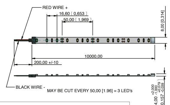
The strip itself and all of its components may not be mechanically stressed. Assembly must not damage or destroy conducting paths on the circuit board. Correct electrical polarity needs to be observed, wrong polarity may destroy the strip. When mounting on a metallic or otherwise conductive surfaces, there needs to be electrical isolation points between strip and the mounting surface. Caution needs to be taken after cutting the strip that exposed ends are insulated.
