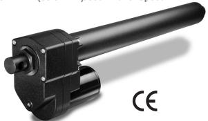
The K2x model provides the highest load rating in its class. This model incorporates all of the base K2 features with a ball nut screw for a 2,800 lb. (1270kg) load capability within a compact package size. The K2x includes a bi-directional wrap spring brake for load holding capability. These units are well suited for the most demanding applications where an alternative to hydraulic or air cylinders is needed or where hydraulic power sources are not available.
