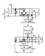
3/2 Single air pilot valve, 1/4"... 1/2" ports Dimensions in mm Projection/First angle
