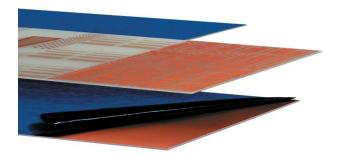
Microtrak FR4 epoxy glass laminates are dip coated with a high resolution positive working Photoresist. The Photoresist contains a dye which gives a good contrast against the copper, allowing boards to be easily inspected at the developing stage. Panels are protected by a specially designed light-proof blue film which allows panels to be guillotined without the risk of fracturing the Photoresist.
