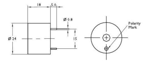
Dimensions Unit: mm Tolerance: ±0.5mm
