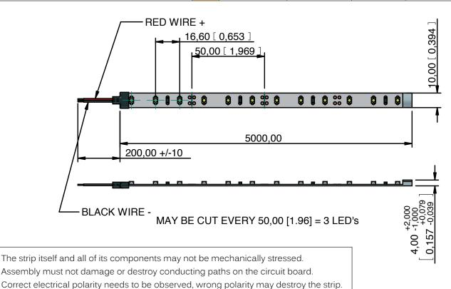
Caution needs to be taken after cutting the strip that exposed ends are insulated.
