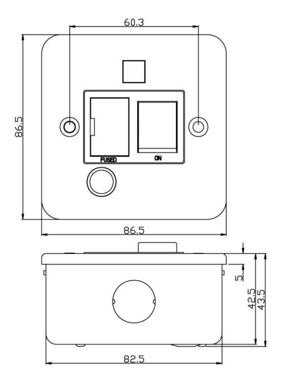
1G SWITCHED FUSED CONNECTION UNIT WITH FLEX OUTLET AND NEON
