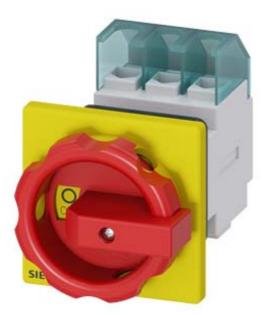
SENTRON, Switch disconnector 3LD, emergency switching-off switch, 3- pole, lu: 25 A, operating power / at AC-23 A 400 V: 9.5 kW, front-mounted, rotary operating mechanism, Red / yellow, central mounting 22.5 mm of the handle
