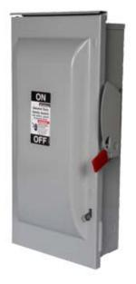
Siemens Low Voltage Circuit Protection General Duty Safety Switches. Type: Safety Switch, Enclosed General Duty Special Features: Non Fusible Application: Construction, Industrial, Residential Std: UL98 V. Rating: 240V A. Rating: 100A No. Of Poles: 3 Action: Single Throw Material: Galvanized Steel Size: H 23.46 x W 11.67 x D 14.68 inches Enclosure: Type 3R Mounting: 2 or 3 Point Mounting Lever O. Cycles: UL 98 Cycles Environmental Conditions: Seismic T58569.01-1
