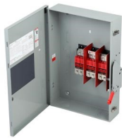
Siemens Low Voltage Circuit Protection Heavy Duty Safety Switch. 3-Pole Non-Fused in a type 3R enclosure (outdoor). Rated 600VAC (400A).
