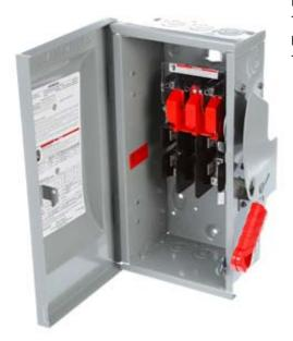
Siemens Low Voltage Circuit Protection Heavy Duty Safety Switches. Type: ENCLOSED, SAFETY SWITCH Std: UL V. Rating: 600V A. Rating: 60A No. Of Poles: 3P F. Rating: 60Hz Action: SINGLE THROW Material: STEEL Enclosure: TYPE 1. 2-3 point mounting holes. O. Cycles: 10000 O. Temperature: (-20F-120F) AMBIENT TEMPERATURE Environmental Conditions: INDOOR
