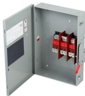
Siemens Low Voltage Circuit Protection Heavy Duty Safety Switch. 3-Pole Non-Fused in a type 1 enclosure (indoor). Rated 600VAC (400A).
