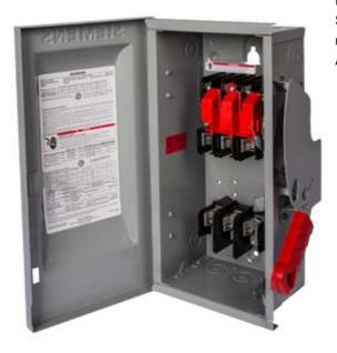
Siemens Low Voltage Circuit Protection Heavy Duty Safety Switches. Type: ENCLOSED, SAFETY SWITCH Std: UL V. Rating: 600V A. Rating: 60A Wattage: 4W No. Of Poles: 3P F. Rating: 60Hz Action: SINGLE THROW Material: STEEL Enclosure: TYPE 1. 2-3 point mounting holes. O. Cycles: 10000 O. Temperature: (-20F-120F) AMBIENT TEMPERATURE Environmental Conditions: INDOOR
