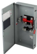
Siemens Low Voltage Circuit Protection Heavy Duty Safety Switch. 2-Pole 2-Fuse and solid neutral Fused in a type 3R enclosure (outdoor). Rated 240VAC (400A).
