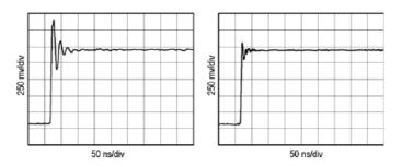
HF transient response with (left) and without (right) extension leads
