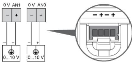
The (-) poles are connected internally.
