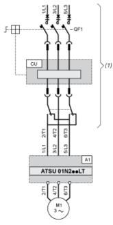
(1) TeSys U with reversing unitA1: Soft start/soft stop unitQF1:TeSys U controller-starterCU: TeSys U control unit
