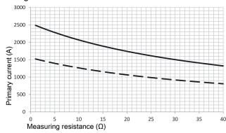
—— U<sub>C</sub> = ±24 V -5 %, T<sub>A</sub> = 85 °C ——— U<sub>C</sub> = ±15 V -5 %, T<sub>A</sub> = 85 °C
