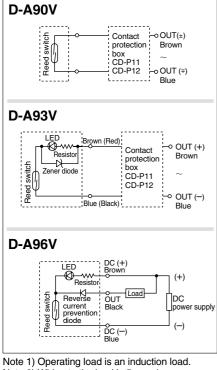
Note 2) Wiring to the load is 5 m or longer.
