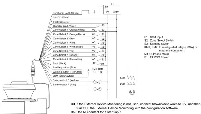
**\*3.**For zone select switch setting, refer to OS32C Series User's Manual (Man.No.Z296-E1). When using only one zone, no connection is needed for the zone select inputs.
