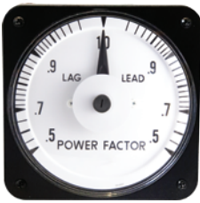
POWER FACTOR SCALE FOR BALANCED SYSTEM
