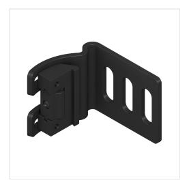
EZ-SCREEN Low Profile Accessory Bracket: Side Mount Includes One Bracket and Hardware Rotation: + 10 Degrees and -30 Degrees 14 ga Steel, Black Zinc Plated Part Number: 82842
