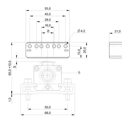
1) not included in scope of delivery, 2) Lateral offset, 3) Distance to BTL
