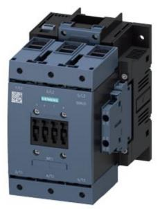
Power contactor, AC-3 115 A, 55 kW / 400 V AC (50-60 Hz) / DC operation 200-277 V UC Auxiliary contacts 2 NO + 2 NC 3-pole, Size S6 with box terminals Drive: electronic with PLC interface 24 V DC screw terminal
