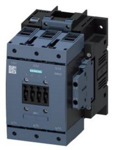
Power contactor, AC-3 115 A, 55 kW / 400 V AC (50-60 Hz) / DC operation 96-127 V UC Auxiliary contacts 2 NO + 2 NC 3-pole, Size S6 with box terminals Drive: electronic with PLC interface 24 V DC screw terminal
