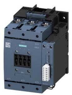
Power contactor, AC-3 115 A, 55 kW / 400 V AC (50-60 Hz) / DC operation 200-277 V UC Auxiliary contacts 1 NO + 1 NC 3-pole, Size S6 with box terminals Drive: electronic with PLC / SIMOCODE interface and RLT signal
