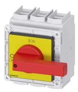
SENTRON, Switch disconnector 3LD, emergency switching-off switch, 3- pole, lu: 160 A, operating power / at AC-23 A 400 V: 75 kW, front-mounted, knob-operated mechanism, red/yellow, 4-hole mounting of the handle
