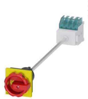
SENTRON, Switch disconnector 3LD, emergency switching-off switch, 4- pole, lu: 16 A, operating power / at AC-23 A 400 V: 7.5 kW, floor mounting with door coupling, rotary operating mechanism, Red / yellow, 4-hole mounting of the handle
