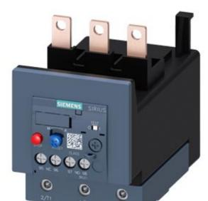
Overload relay 70...90 A Thermal For motor protection Size S3, Class 10 Contactor mounting Main circuit: Screw Auxiliary circuit: Screw Manual-Automatic-Reset
