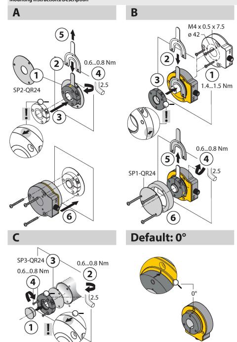
Extensive range of mounting accessories for easy adaptation to many different shaft diameters. Based on the functional principle of RLC coupling, the sensor operates absolutely wear-free and is immune to magnetized metal splinters and other interference fields. Wrong installation is hardly possible.
