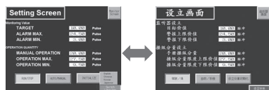
Example: The label switch function can be used to switch between English and Simplified Chinese.
