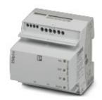
Multi-functional energy measuring device without display with direct Rogowski connection and integrated Modbus/TCP and PROFINET interface for measuring electrical parameters in low-voltage installations up to 690 V
