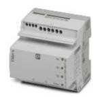
Multi-functional energy measuring device without display with integrated Modbus/TCP and EtherNet/IP™ interface for measuring electrical parameters in low-voltage installations up to 690 V.
