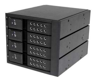
The HSB4SATSASBA Removable 4-drive Backplane makes inserting and removing drives fast and easy, by turning three 5.25" bays into a hot-swappable interface for up to four 3.5" SATA or SAS hard drives (HDD).
