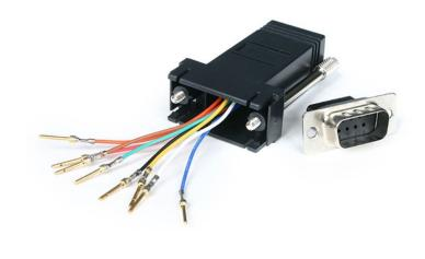
The GC98MF Modular Adapter features a DB9 male connector and an RJ45 female connector. Used for modular RS232, RS422 and RS485 connections, the adapter converts your DB9 female connection into an RJ45 female connection. The adapter allows for custom serial pin out configurations.
