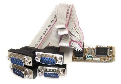
The MPEX4S952 4-Port RS232 Mini PCI Express Serial Card (16650 UART) turns a mini-PCIe slot into four RS232 (DB9) serial ports with data rates up to 921.6 Kbps - a cost-saving solution for adding serial support to embedded systems missing the functionality.
