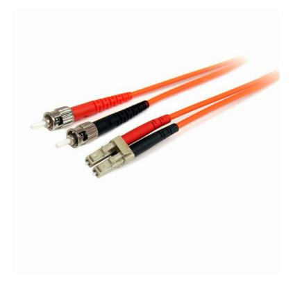
The FIBLCST5, 5-meter (16ft) Multimode 62.5/125 Duplex Fiber Patch Cable is terminated with one LC (male) connector and one ST (male) connector, to provide the necessary connection between fiber networking devices for high-speed, long distance networks.
