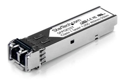
The SFPGESST is a Cisco SFP-GE-S compatible fiber transceiver module that has been designed, programmed and tested to work with Cisco® brand switches and routers. It delivers dependable 1 GbE connectivity over fiber cable, for 1000BASE-SX compliant networks, with a maximum distance of up to 550 m (1804 ft).
