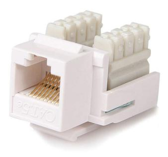
This Cat5e RJ45 Keystone Jack snaps into a wall plate, enabling mixed media outlets to adapt television cable and Ethernet (10BaseT, 100BaseT and 10Base2) cabling.
