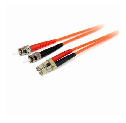
The FIBLCST1 1-meter (3.3ft) Multimode 62.5/125 Duplex Fiber Patch Cable is terminated with one LC (male) connector and one ST (male) connector, to provide the necessary connection between fiber networking devices for high-speed, long distance networks.
