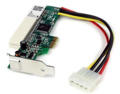
This PCIe to PCI Adapter Card lets you use low profile PCI expansion cards in a server or desktop motherboard PCI Express slot. Compliant with PCI Express Specification 1.0a and PCI Specification 2.2, the adapter card connects through a PCIe 1x slot to provide a low profile PCI slot in its place. A spare full size bracket for PCI Express card is also included for use in larger desktop or server PCI Express slots.
