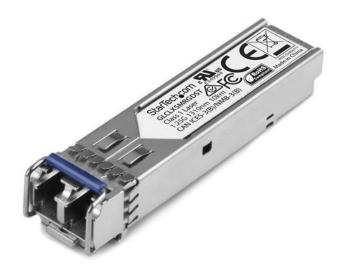
The GLCLXSMRGDST is a Cisco GLC-LX-SM-RGD compatible fiber transceiver module that has been designed, programmed and tested to work with Cisco® brand switches and routers. It delivers dependable 1 GbE connectivity over fiber cable, for 1000BASE-LX compliant networks, with a maximum distance of up to 10 km (6.2 mi).
