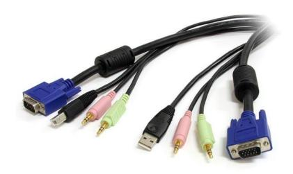
The USBVGA4N1A6 6 ft 4-in-1 USB VGA KVM Switch Cable with Audio and Microphone provides VGA video, USB mouse and keyboard, 3.5mm audio, and 3.5mm microphone connections, all in a single, compact cable.
