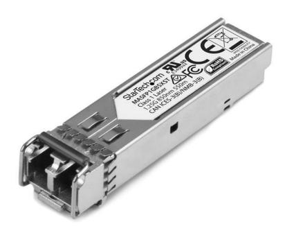
The MASFP1GBSXST is a Cisco Meraki MA-SFP-1GB-SX compatible fiber transceiver module that has been designed, programmed and tested to work with Cisco Meraki<sup>™</sup> brand switches and routers. It delivers dependable 1GbE (1000 Mbps) connectivity over fiber cable, for 1000BASE-SX compliant networks, with a maximum distance of up to 550m (1804 ft).
