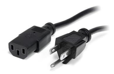
The PXT101143 NEMA 5-15P to C13 Computer Power Cord (3ft) features 14 AWG wire suitable for high power connections, making it a reliable solution for large server applications that require a higher rated, heavier gauge cable, and connecting to Power Distribution Units (PDU).
