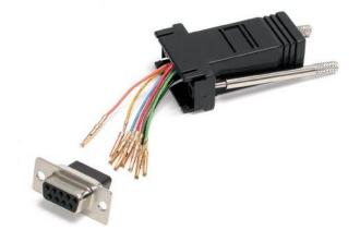
The GC98FF Modular Adapter features a DB9 female connector and an RJ45 female connector. Used for modular RS232, RS422 and RS485 connections, the adapter converts your DB9 male connection into an RJ45 female connection. The adapter allows for custom serial pin out configurations.
