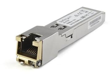
The RXGETSFPST is a Juniper RX-GET-SFP compatible copper transceiver module that has been designed, programmed and tested to work with Juniper brand switches and routers. It delivers dependable 1 GbE connectivity over copper cable, for 1000Base-T compliant networks, with a maximum distance of up to 100 m (328 ft).
